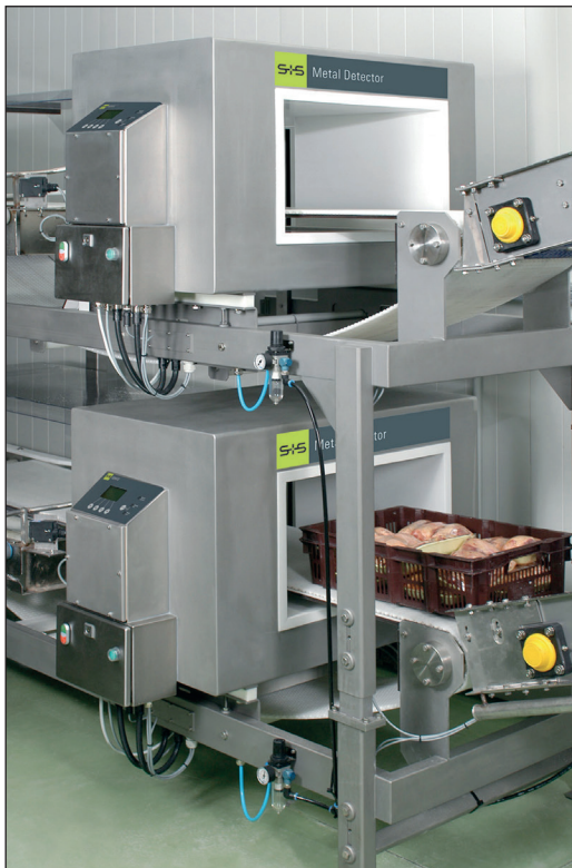
Metal inspection of poultry in E1 containers
